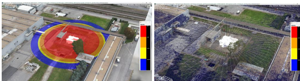
Figure B.1.3 a) Example of risk contours according to Italian regulation (see [D16]); b) example of calculation grid adopted for triangularization of circular areas.
