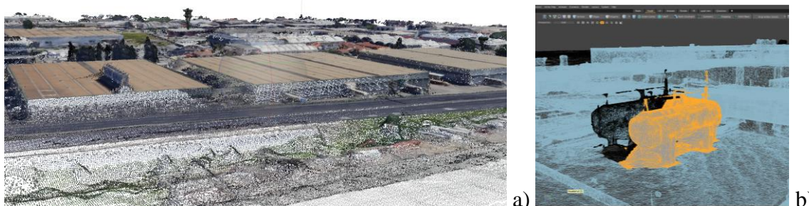
Figure B.1.1: a) Example of polygonal 3D model with textures created with Agisoft Metashape; b) detail of the LPG tank at DEMO2.
