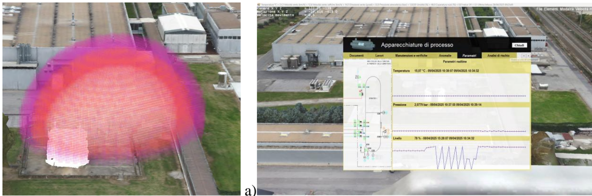
Figure B.1.2 a) Example of polygonal 3D model with textures created with Agisoft Metashape; b) Example of real time data extracted from DEMO2 (Temperature, pressure, level).
